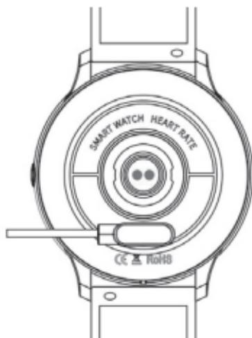
\*Be aware that the two contacts of the USB cable are not allowed to contact the conductor at the same time, or it will cause the circuit to burn.
